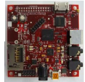
600MHz Cortex-A8 based Beagleboard No fan or heat sink required.
